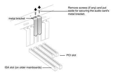
Figure 2-2: Removing metal brackets
